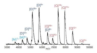
The higher mass quadrupole also improves transmission performance for higher masses in general. This provides you with sufficent sensitivity to detect also less abundant isoforms
