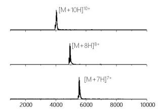
The soft selection and transmission of the MS Vision quadrupole also ensures the preservation of non-covalent interactions for native mass spectrometry.
